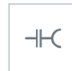
Capacitive voltage detection system
